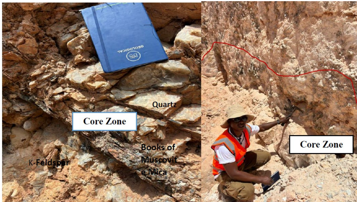
Figure 5. Shows the Core of the opened pegmatite showing Quartz crystals, books of Muscovite micas and K-feldspar with matrix of Albite feldspar.
