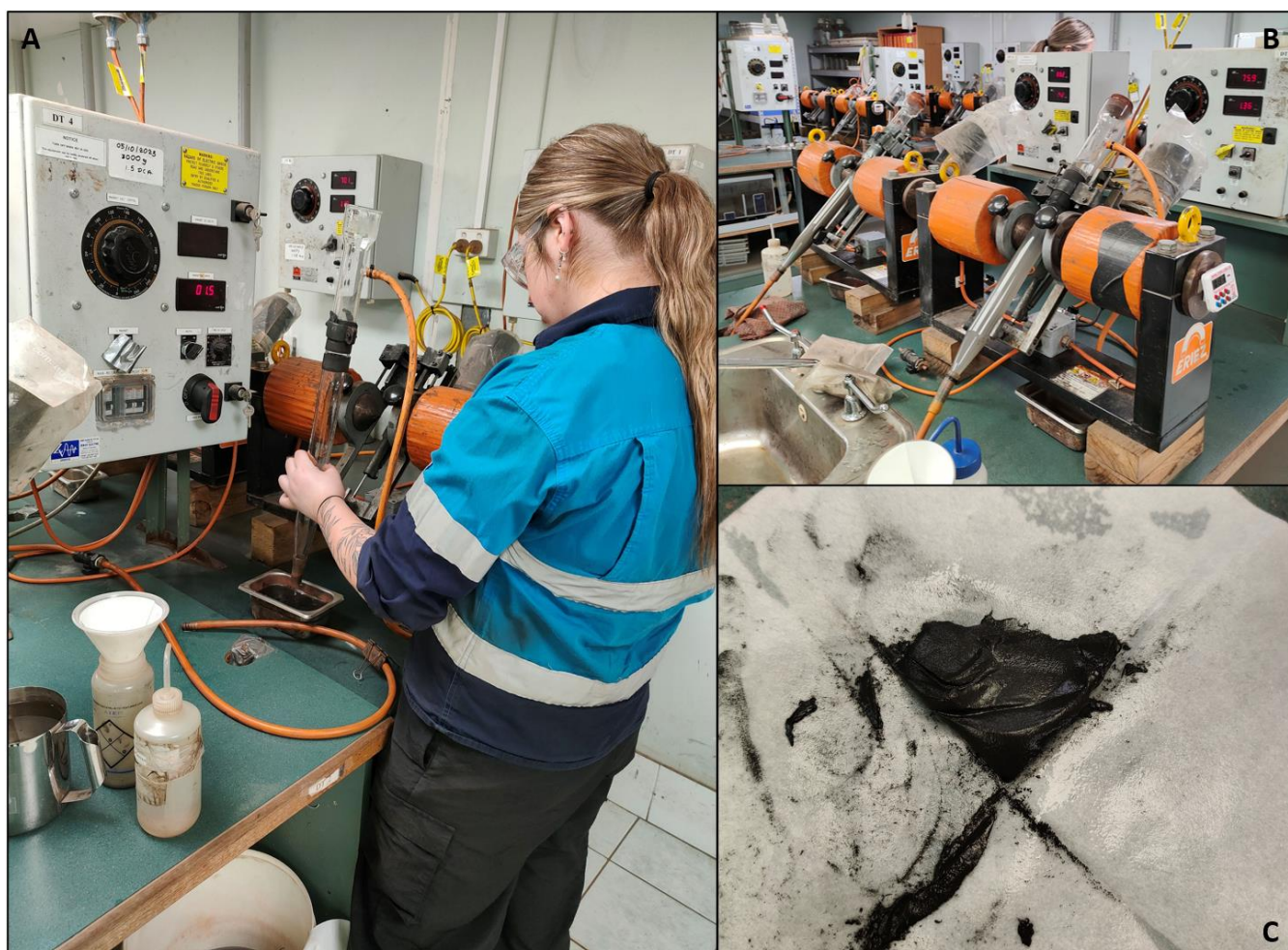
Figure 3; Photos showing A) Samples being prepared for filtration after DTR testwork completed, B) Eirez Davis Tube tester setup for sighter DTR testing and C) Magnetic concentrate produced after filtration.
