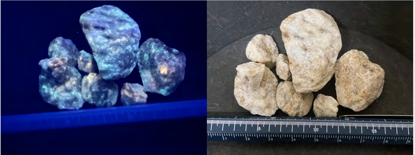
Figure 4. Pegmatite chips obtained from drill spoil at an historical Bullion Minerals RAB drill collar LJR010. Photograph taken under a long wave ultraviolet (UV) light source (left), and natural light (right). Scale bar is in centimeters.
