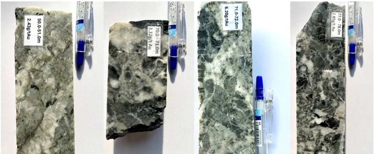
Figure 3: Silicified hydrothermal breccia in 7726DD, assayed up to 6.20 g/t Au and 124 ppm Ag.
