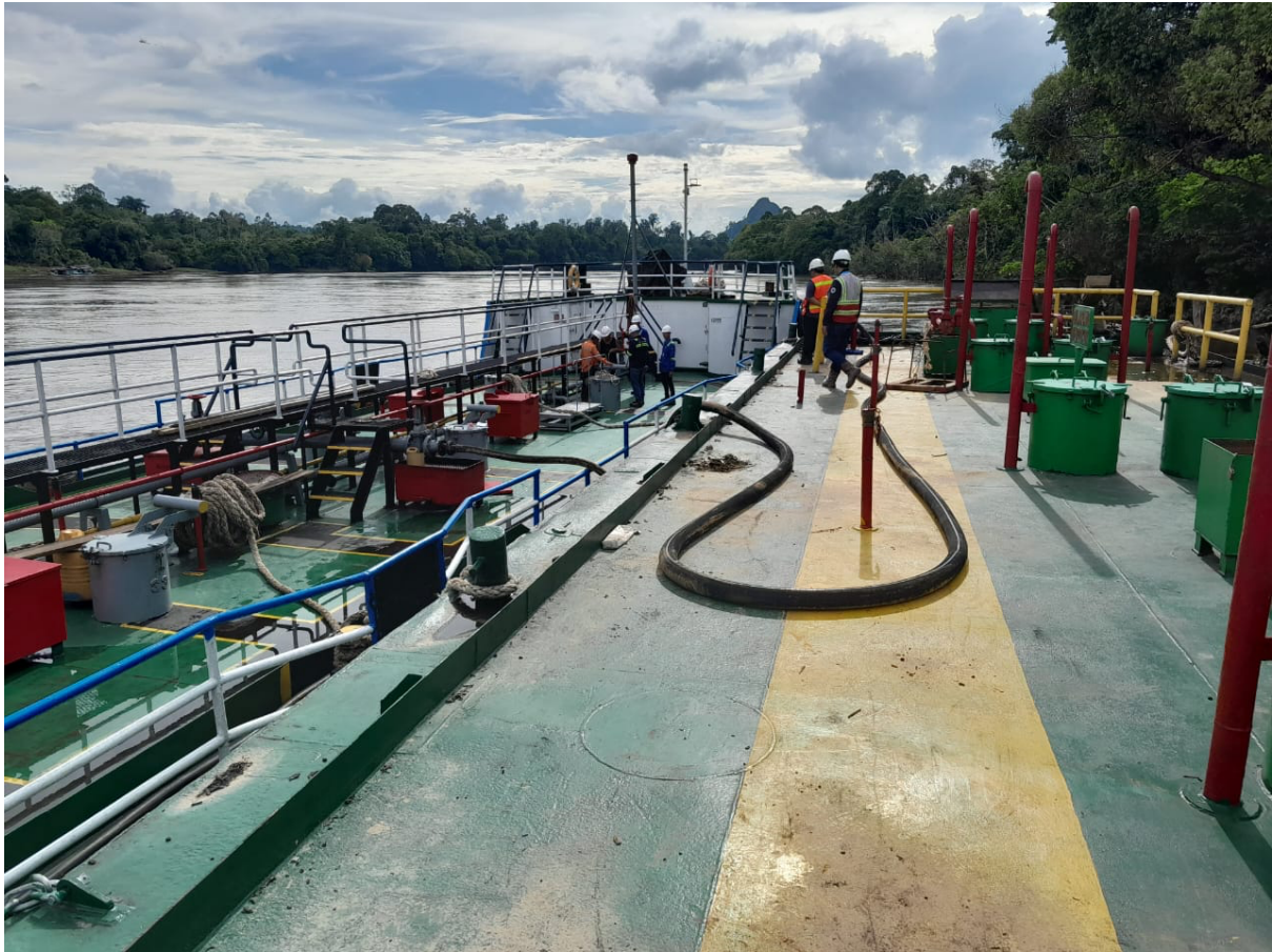
Fuel transfer from bunker barge to floating storage at Batu Tuhup Jetty
