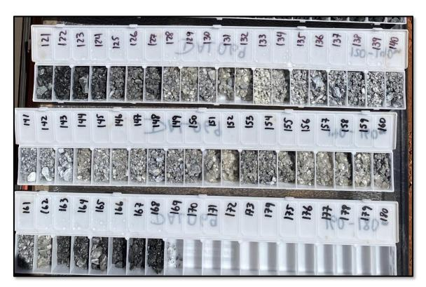
Figure 1 Photograph of drill hole DAL069 chip tray showing 39m intersection of pegmatite
