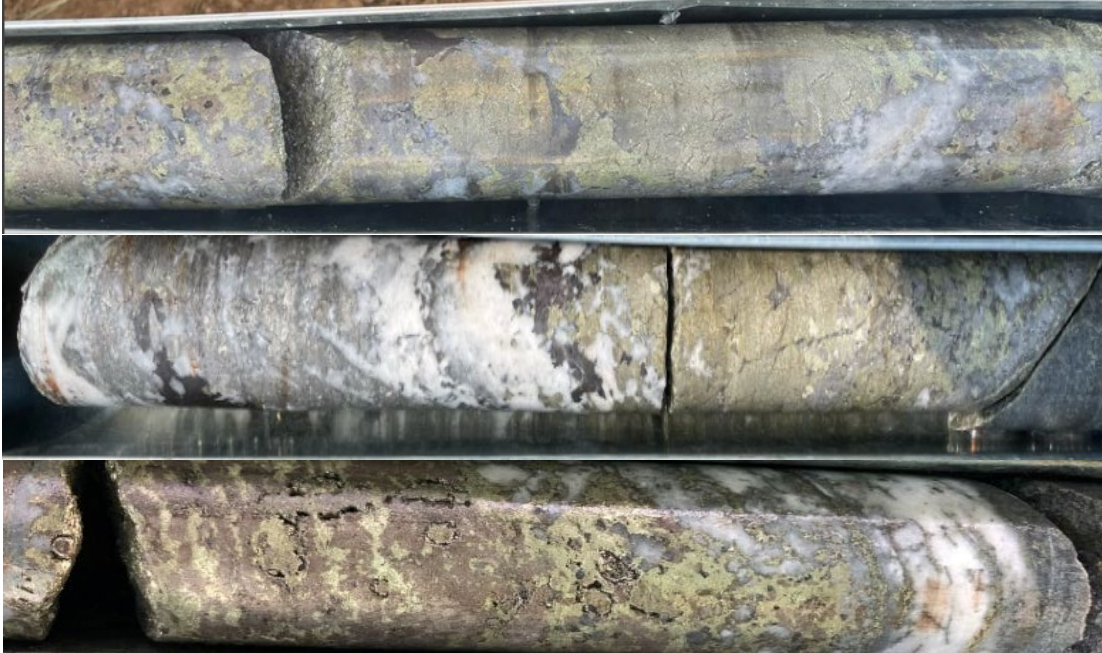
Figure 4 | Mineralised veins in Memot Diamond Core. Quartz veining with Pyrite, Arsenopyrite, Pyrrhotite, Chalcopyrite and Sphalerite sulphides. Top: DD22MMT080W – 0.6m @ 31.60g/t Au, 6.04% Cu, 0.16% Pb and 0.25% Zn from 192m Middle: DD22MMT013 - 0.4m @ 17.70g/t Au, 230g/t Ag, 2.78% Cu, 0.56% Pb and 1.74% Zn from 190m Bottom: DD21MMT006 – 1m @ 25.4g/t Au, 73g/t Ag, 1.81% Cu, 0.1% Zn from 30m
