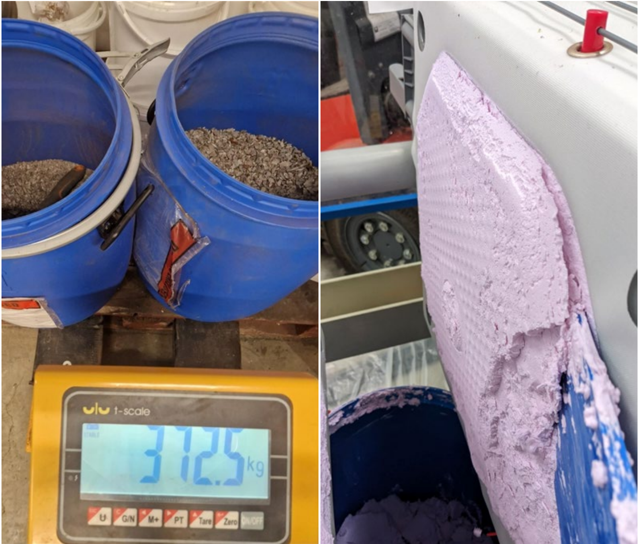
Figure 5: Left, crushed magnets prepared, and right, mixed rare earth filter cake prepared for downstream process commissioning activity.
