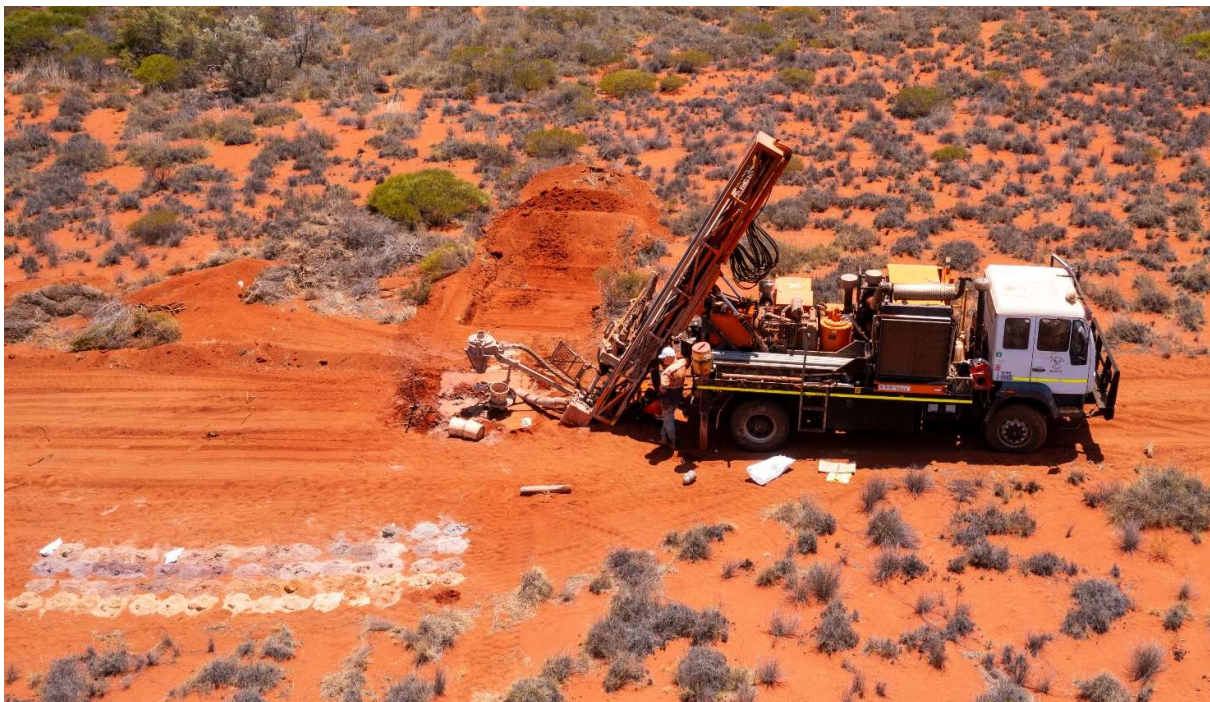
Figure 1. Aircore Drill Rig During the Recently Completed Drill Program
