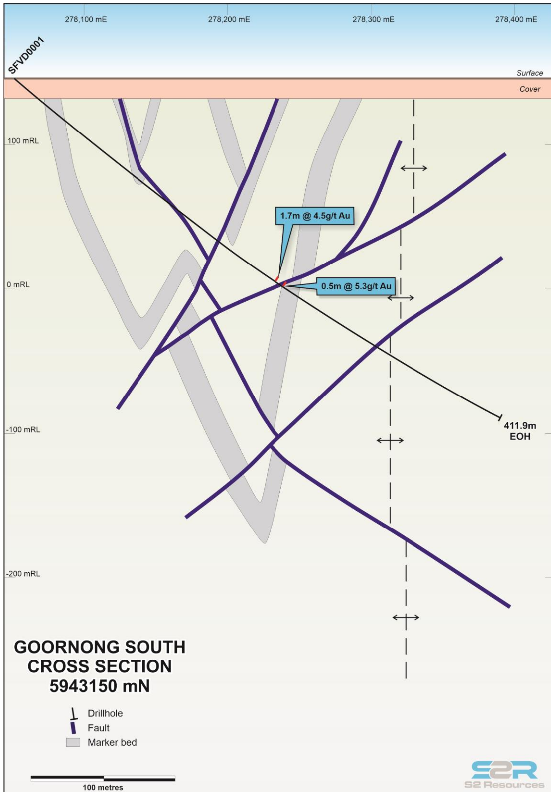
Figure 2. Cross section of the Goornong South area showing drill hole SFVD0001 that tested the favourable anticlinal hinge zone south of the oxide gold mineralisation.
