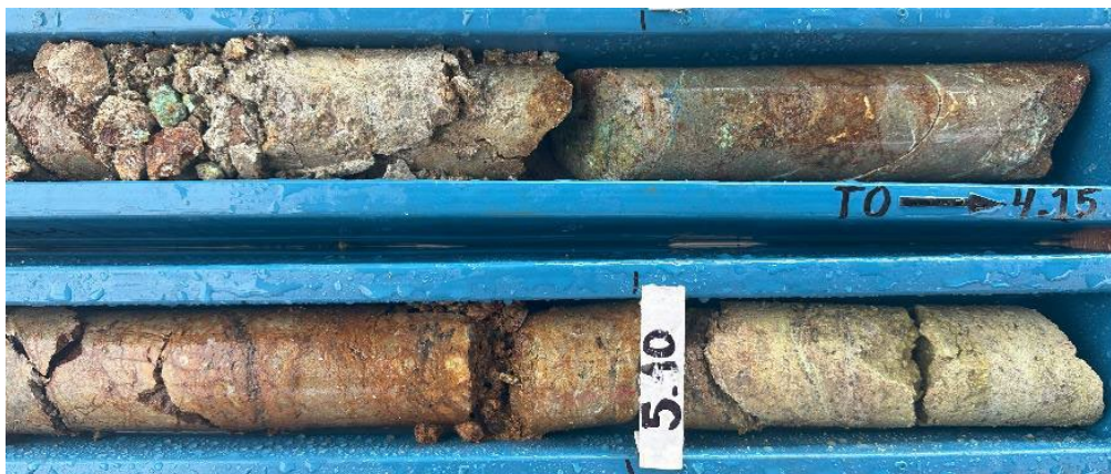
Figure 5: Example of secondary copper mineralisation at around 4-5m depth at Cumbre Coya Target 23PCCD0001
