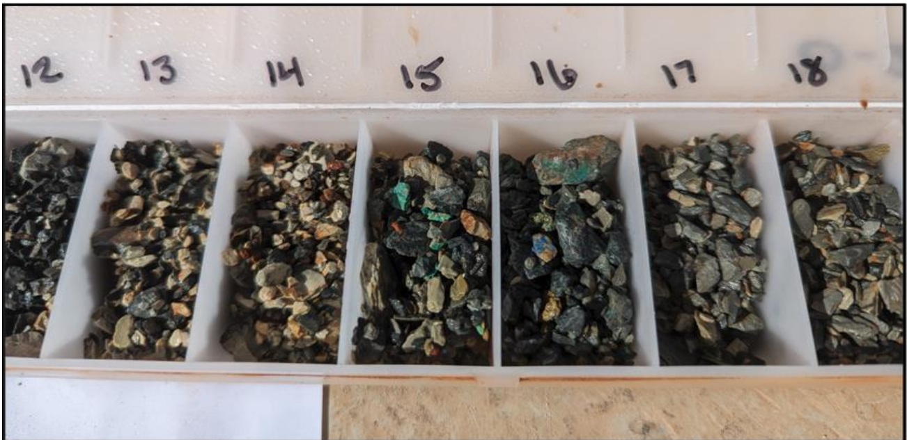
Figure 4 – Chip tray showing BRC004 copper oxide intersection samples (3m @ 6.2% Cu from 13m) with copper oxide minerals malachite and azurite clearly visible.
