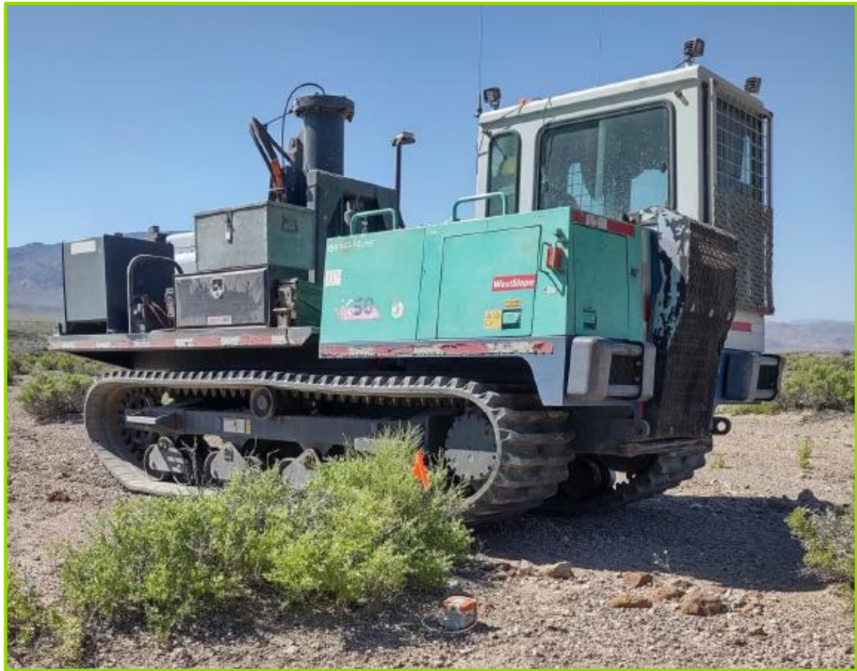
Figure 2: Accelerated weight drop seismic survey source.
