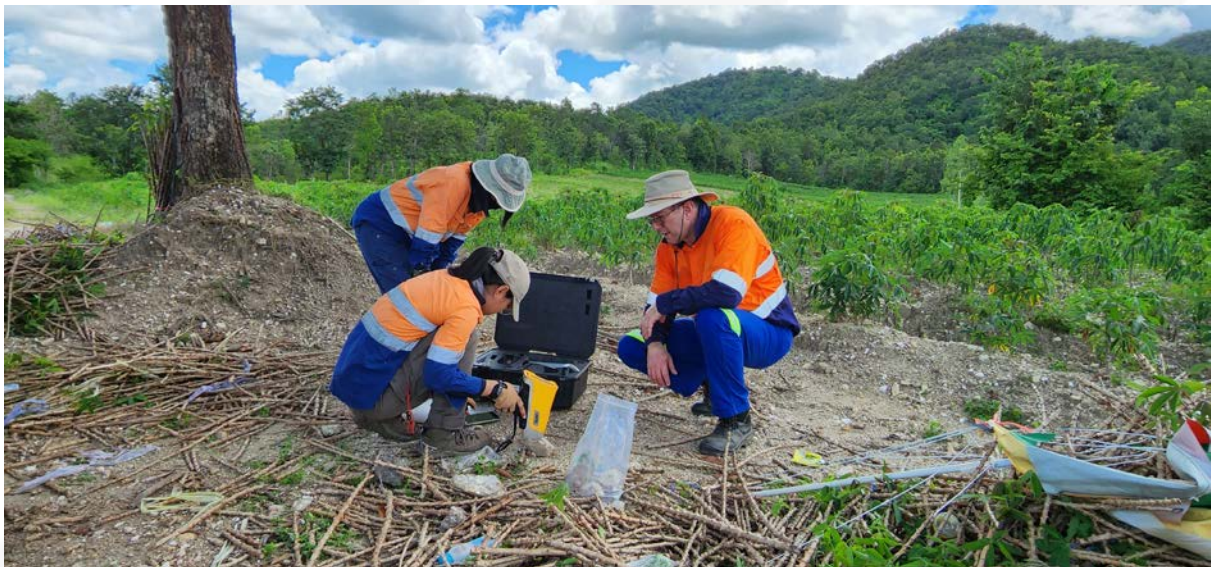
Real time analysis of samples using handheld LIBS analyser to determine fertility of pegmatite occurrences
