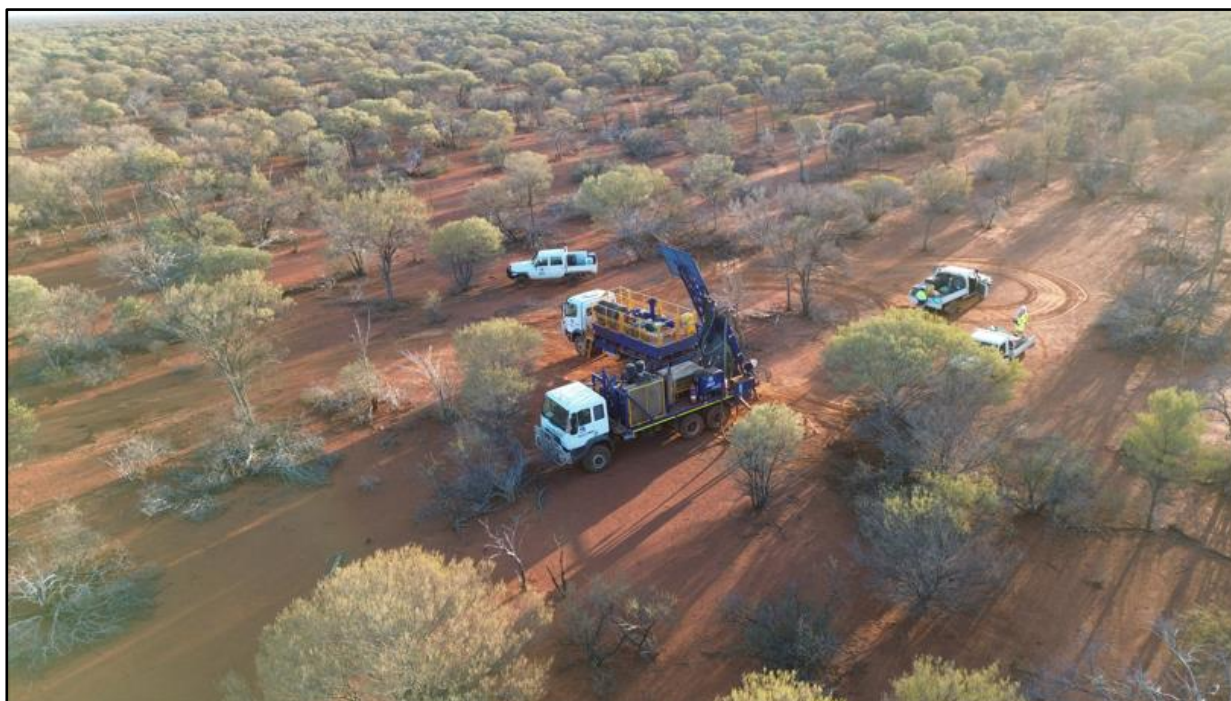
Figure 7: Aircore geochemical drilling in typical soil-covered terrain at the Yarri Project. Extensive soil cover means that any previous surface geochemical sampling can be considered to be largely ineffective.
