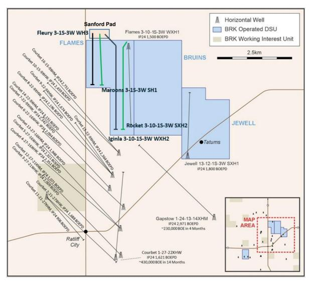
Figure 2: Location of the Sanford Pad and the four FMDP wells: Fleury, Maroons, and Iginla Wells (to be drilled from the Sanford Pad), and the Rocket Well (to be drilled from the existing Flames Well pad). Also shown are Continental Resources Courbet Wells full field development showing the strong performance of both the Woodford wells (well names ending with HXW) and Sycamore wells (well names ending in HXM).
