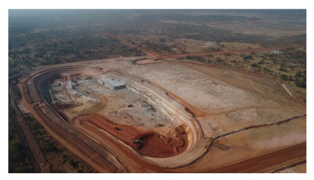
Image 1 – Aerial view of Starter Pit and topsoil clearing of the next cutback
