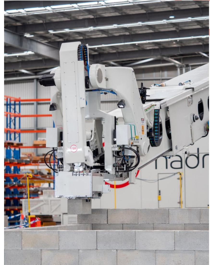
Next-generation Hadrian X ® builds test structure with lay-path vectoring to close perpendicular gaps
