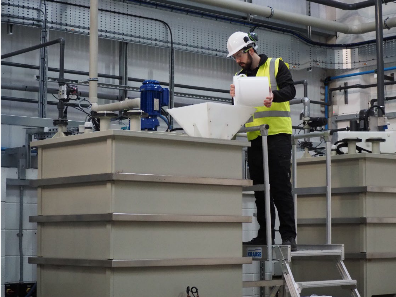
Figure 4: Loading milled magnet slurry into the Digestion reactor.
