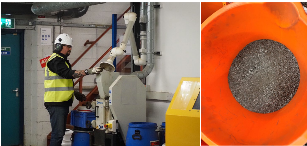
Figure 1: Magnet pre-processing, showing jaw crusher in use on left, and crushed permanent magnets on the right.
