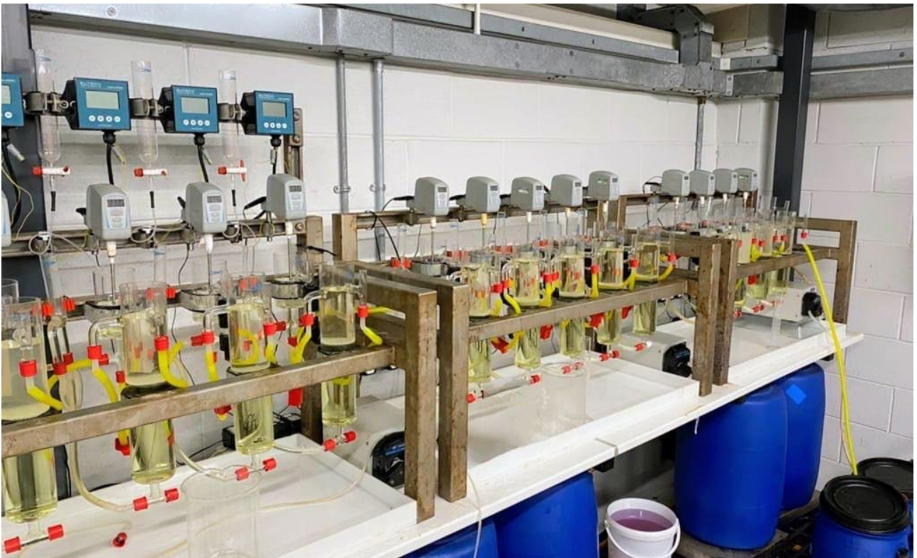
Figure 7: Pilot plant mixer-settler circuit commencing for Dy/Tb separation.
