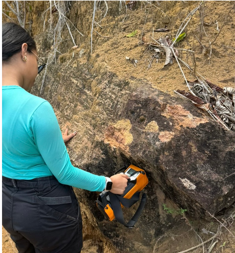
Figure 4: BRE geophysics team conducting gamma spectrometry on hard rock outcrops in Site 2
