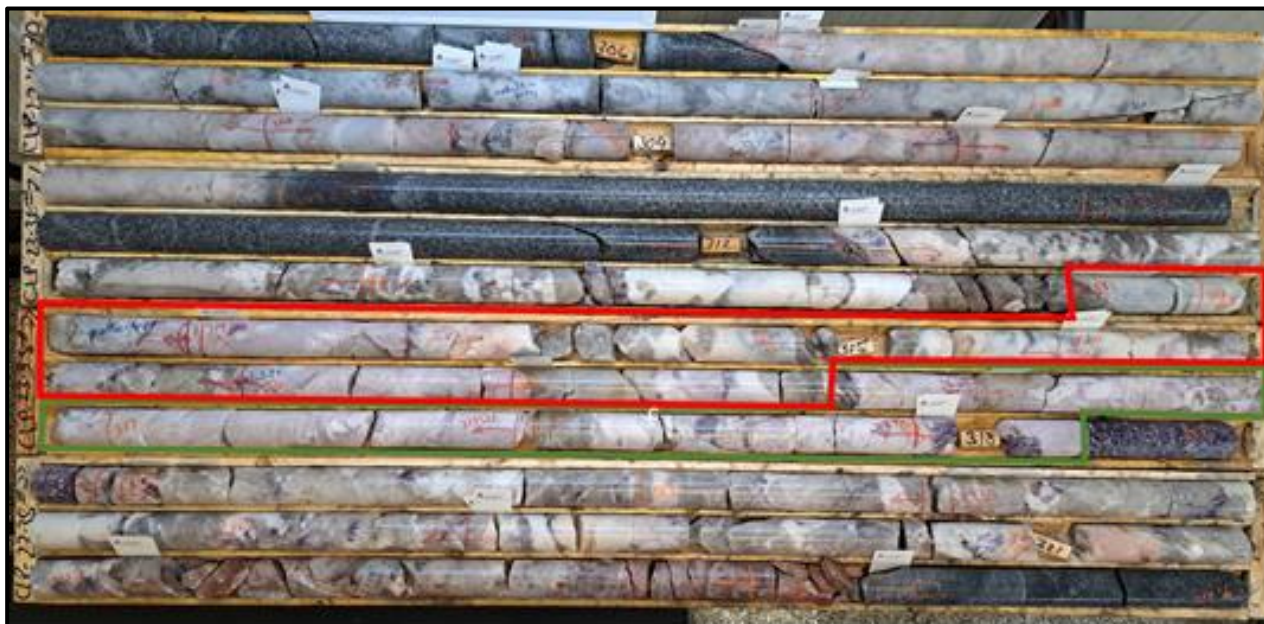
Photo 1: Core from Hole CLP-038 exhibiting pollucite (red outline) and spodumene mineralisation (green outline) between 313m and 318m. Assay results from hole 38 reported 2.9m at 6.8% Cs 2 O and 5.3m at 2.3% Li 2 O.
