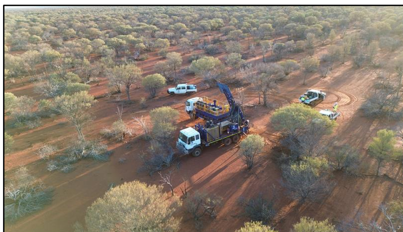
Figure 11: Aircore geochemical drilling in typical soil-covered terrain at the Yarri Project. Extensive soil cover means that any previous surface geochemical sampling can be considered to be largely ineffective.
