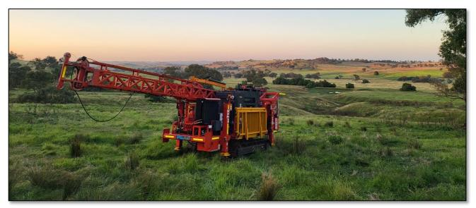
Figure 1: Diamond drill rig collaring hole SPD001 at the Spur Prospect
