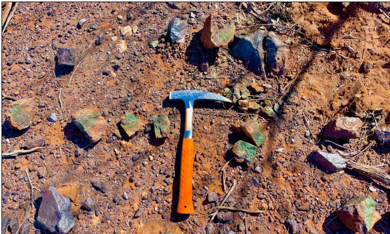
Figure 2. Copper-platinum-palladium-gold-mineralised gossan at Hyperion Reef, Dante Project (refer Table 3).
