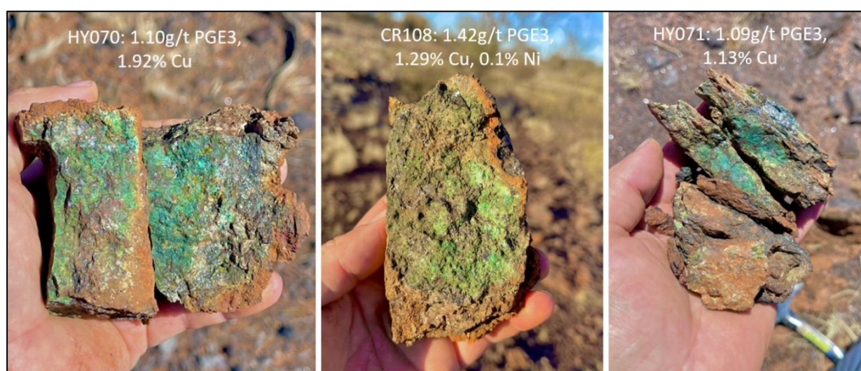
Figure 1. Images of copper-gold-PGE bearing gossans from the Dante Project's PGE reefs
