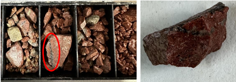
Figure 4. Trace molybdenite (blackish mineral) within quartz stringers (red oval) hosted in microgranite.
