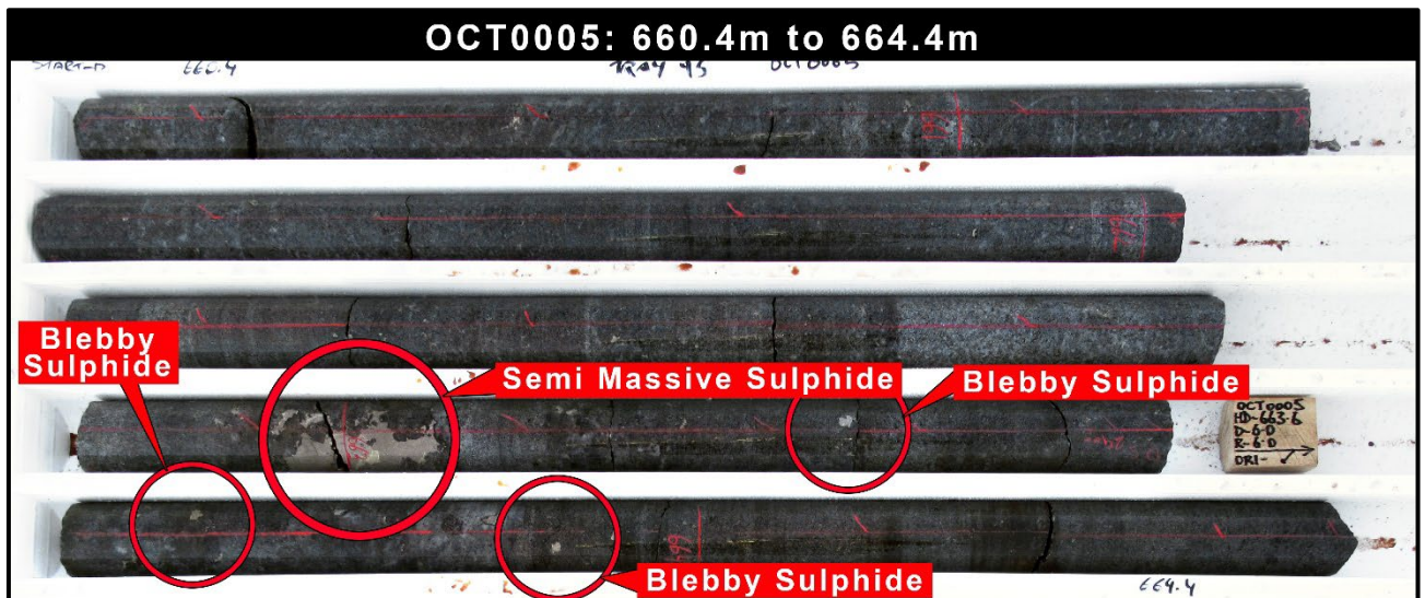
Photo 1: Diamond drill core tray from OCT0005 with visual Ni-Cu sulphide mineralisation. OCT0005 intersects the top edge of conductor 2 .
