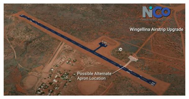
Figure 11. New proposed code 4C airstrip
