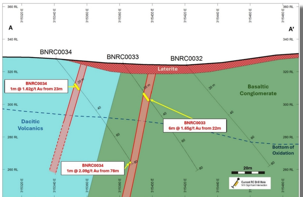
Figure Thirteen | Bouake North Cross Section of Drilling Testing New Gold & Arsenic Anomalism Along a Lithological Contact
