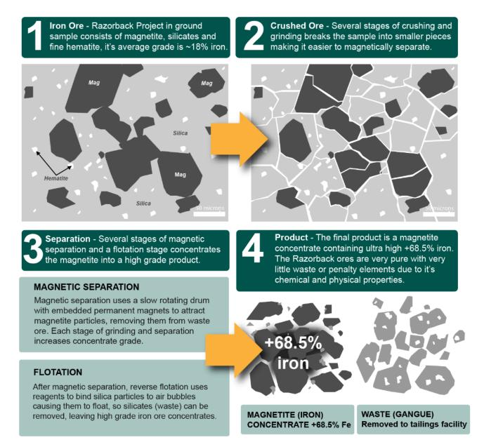
Figure 7. Simplified description of Razorback magnetite liberation and processing into a concentrate
