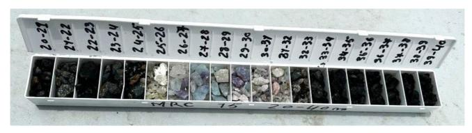
Figure 2: Chip-tray of 20m-40m interval of MRC15.1
