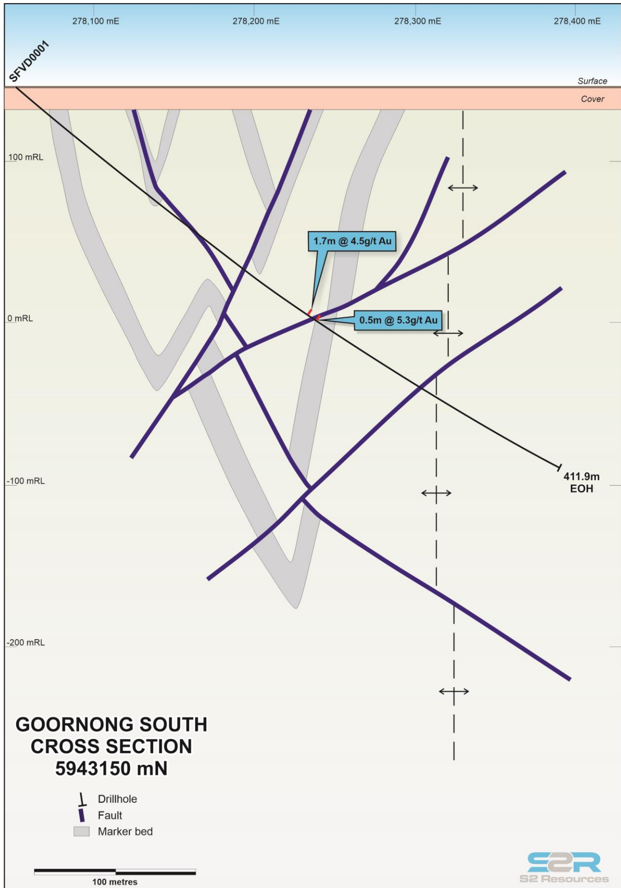
Figure 3. Cross section of the Goornong area showing gold oxide mineralised zone, favourable anticlinal hinge zone, previous ineffective Kirkland Lake holes, and target zones where structures potentially intersect the hinge zone, refract and flatten out, and dilate, to create stacked favourable sites for gold mineralisation (see S2 ASX announcement of 30 th October 2023).
