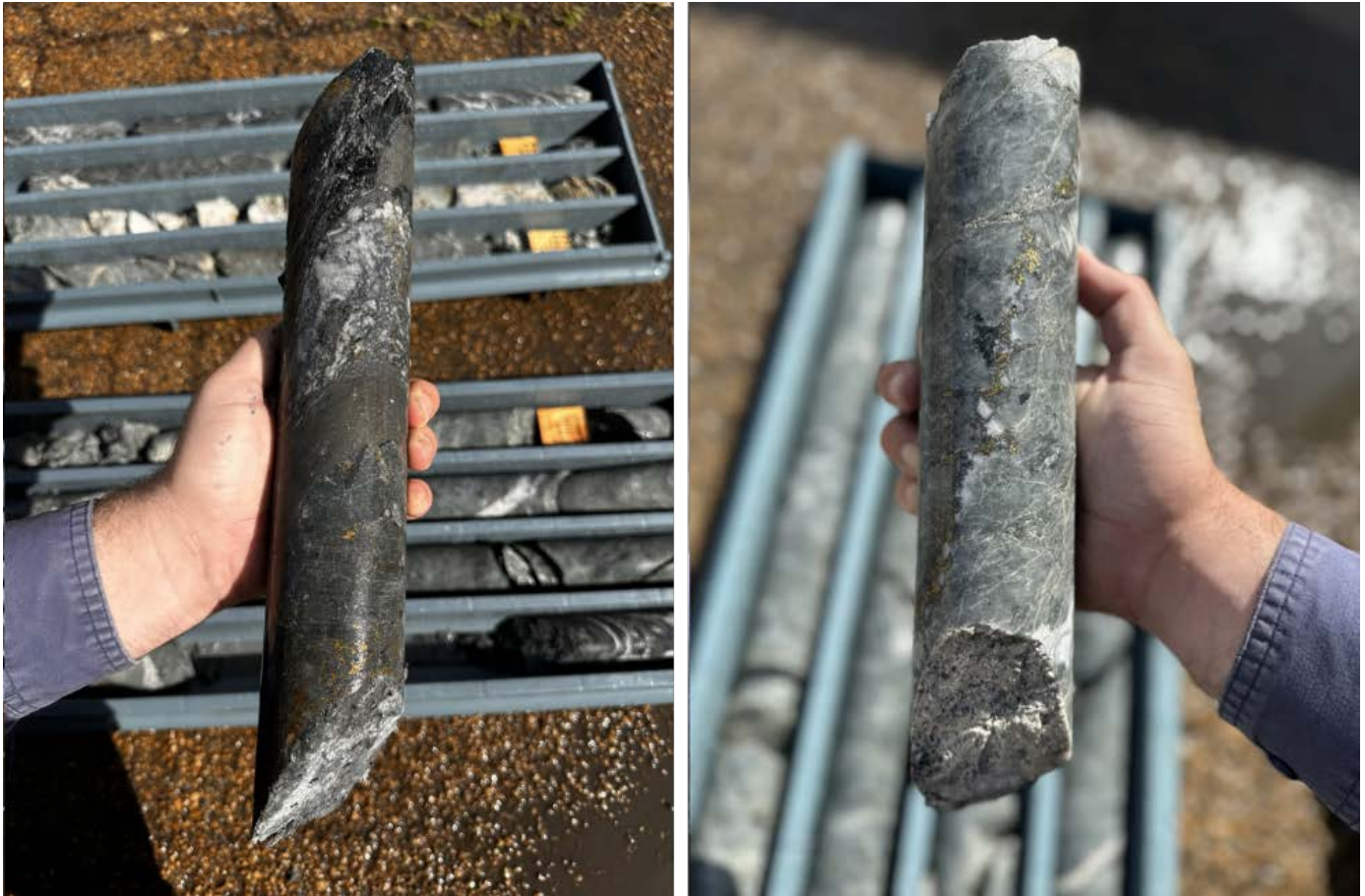
Figure 6. Drill core from 23LTRD001 showing chalcopyrite, sphalerite and barite at 109m from a zone grading 2m @ 3.84 g/t Au, 0.45% Cu, 4.43% Zn (left) and chalcopyrite within a heavily silicified and brecciated volcanic at 116.4m (right).
