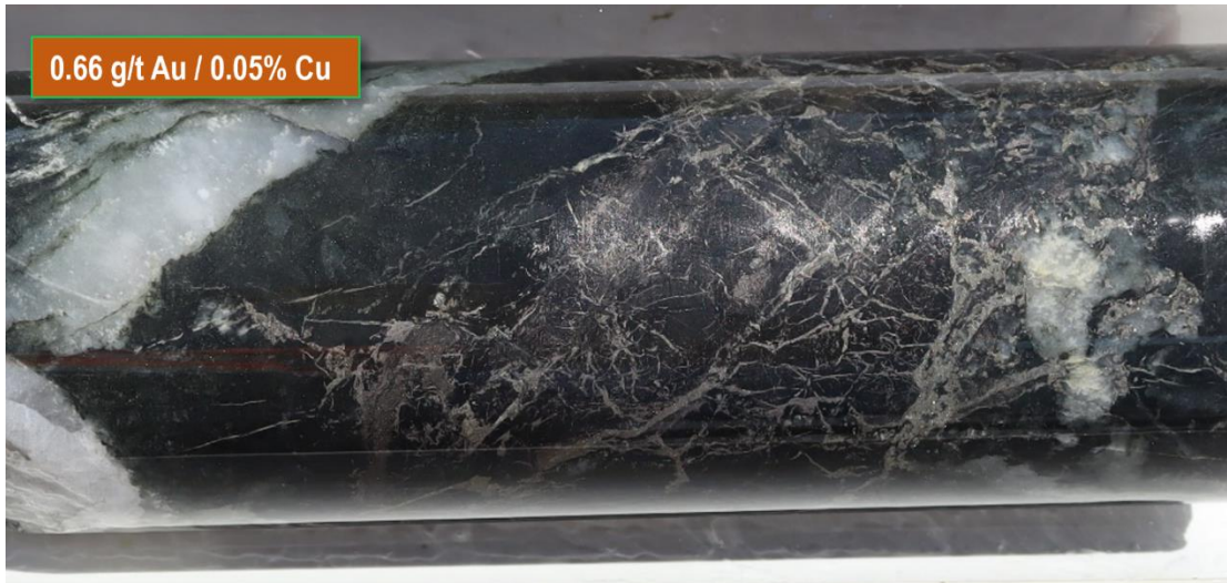
Figure 7: Mineralised Larramore core from hole 23LMDD010 (83.98-84.30m core interval) within an assayed sample length of 83.5 to 84.04 (0.54m) returning 0.66 g/t Au and 507 ppm Cu.
