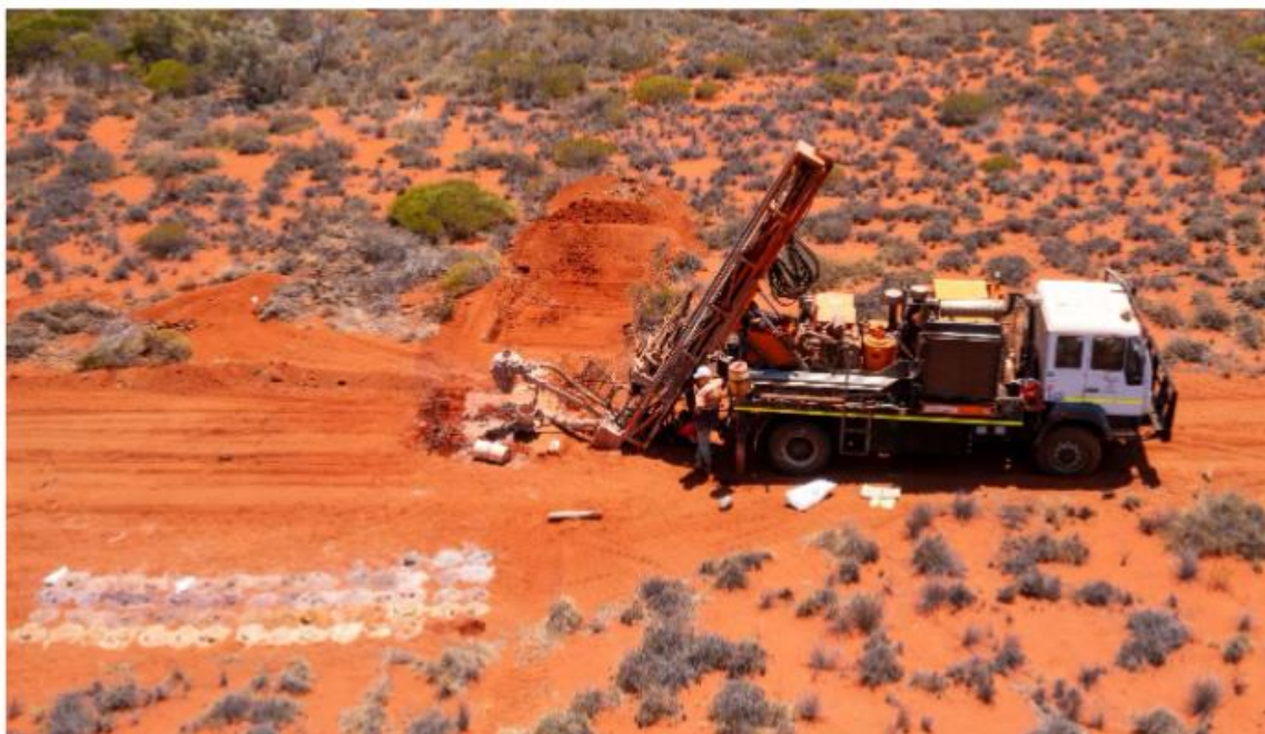
Figure 2: Aircore drill rig during the completed drill program
