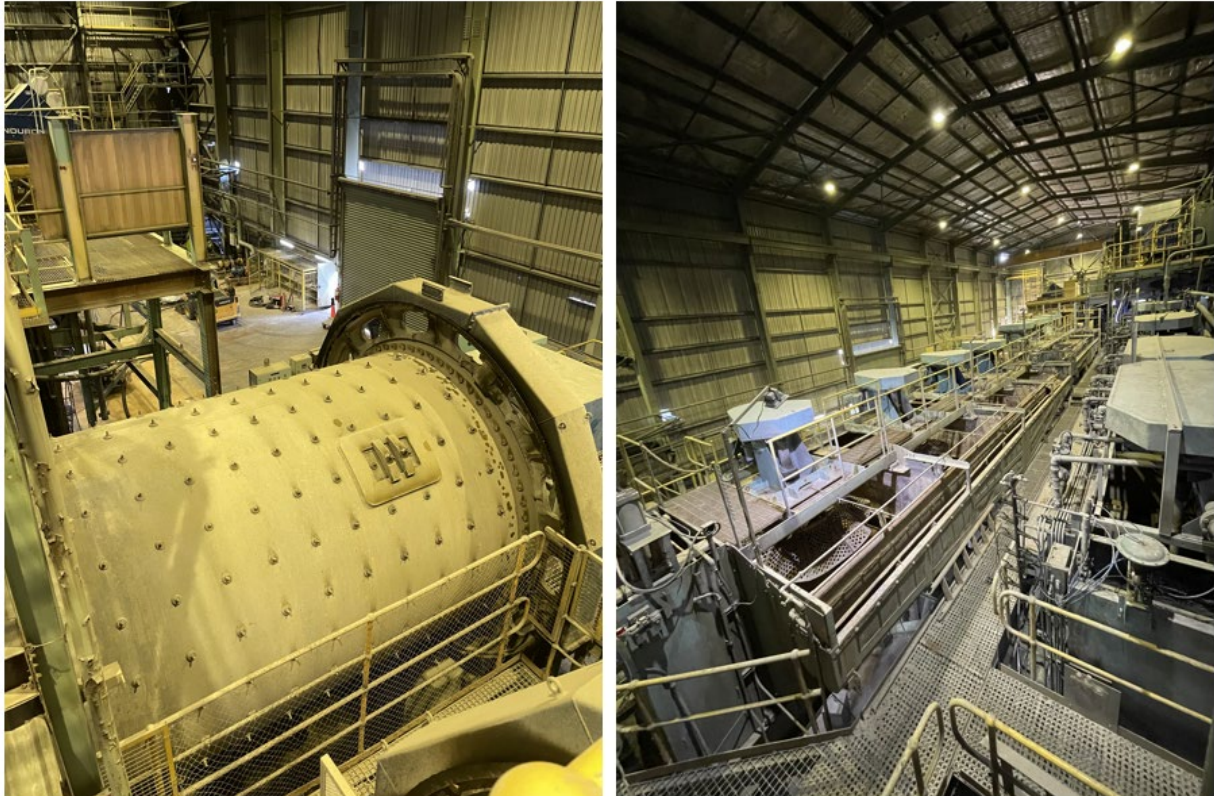
Figures 5: Ball mill and rougher/cleaner/scavenger units in mill.
