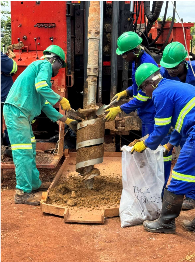
Figures 1 & 2: Bulk sample mechanised spiral drilling and sampling at Kasiya in November 2023
