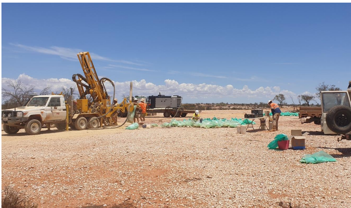
Photo 3. Air Core drill rig at the Bellagio Gold Prospect, with the main quartz vein outcrop shown to the right of the drill rig in the distance, in the direction looking towards the Geologist at the Table. Overall photo direction looking west-southwest.
