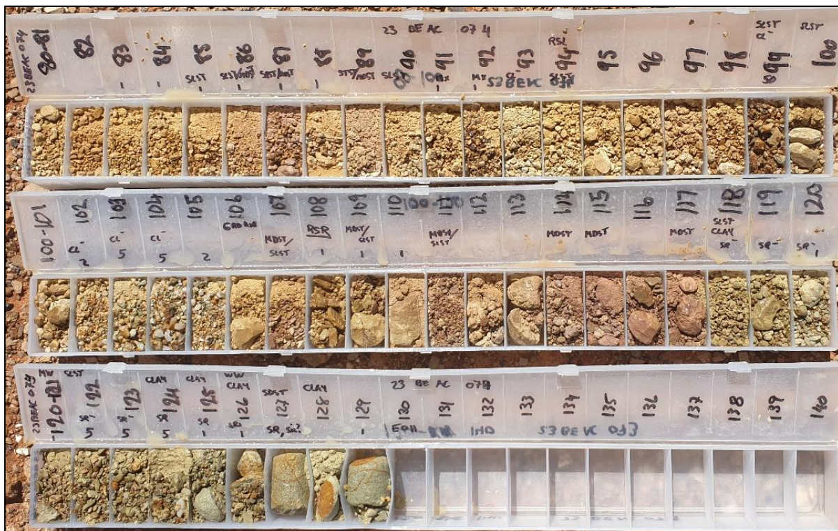
Photo 2. Chip trays from deepest portion of hole 23BEAC074, showing Lower Saprolite (RSL) and Saprock (RSR) boundaries, with Silica-sericite alteration (SR = Sericite) towards the bottom of hole.
