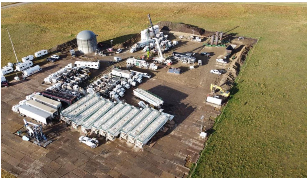
Figure 1. Aerial view of fracture spread on location at the Certus Caroline 1-27-33-05-W5 well.
