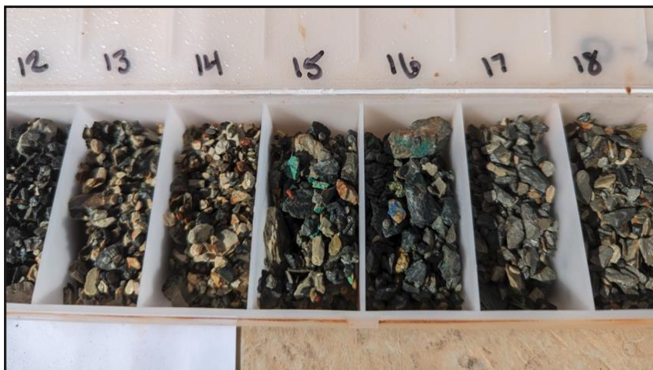
Figure 4 – Chip tray showing BRC004 copper oxide intersection samples (3m @ 6.2% Cu from 13m) with copper oxide minerals malachite and azurite clearly visible.
