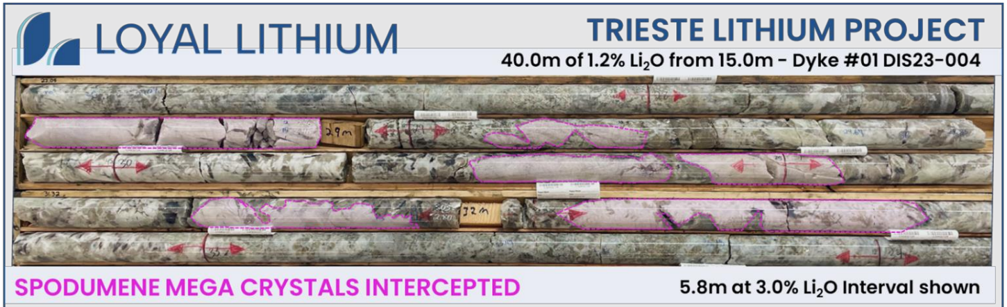
Photo 1: Trieste Lithium Project Multiple Spodumene MEGA Crystals (shaded pink) in drill core DIS23-004.
