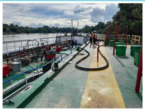
Fuel transfer from bunker barge to floating storage barge Mandiri at Batu Tuhup Jetty under VMI arrangement
