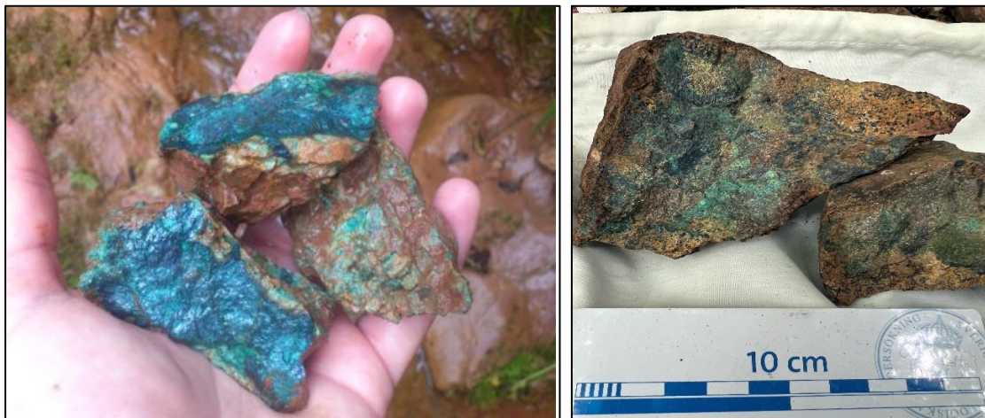
Figure 5 - Sample REG-104923: 20% Cu and 1540ppm – displaying massive chalcocite, azurite and malachite (LHS) and ST008: 6.5% Cu and 155ppm Ag displaying malachite and azurite in sandstone.
