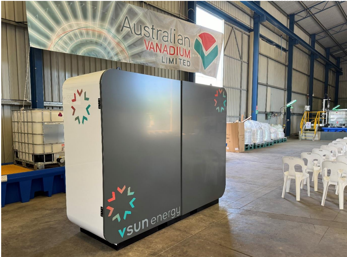
Figure 4 - VSUN Energy prototype residential vanadium flow battery
