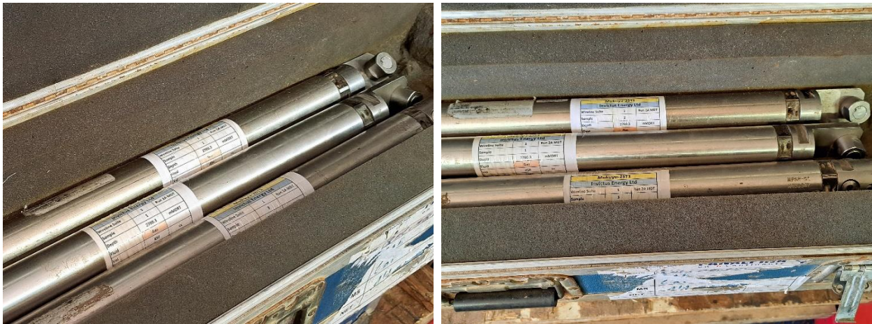
Figure 3 - Downhole gas samples recovered to surface in pressurised chambers in preparation for shipment to the lab for analysis
