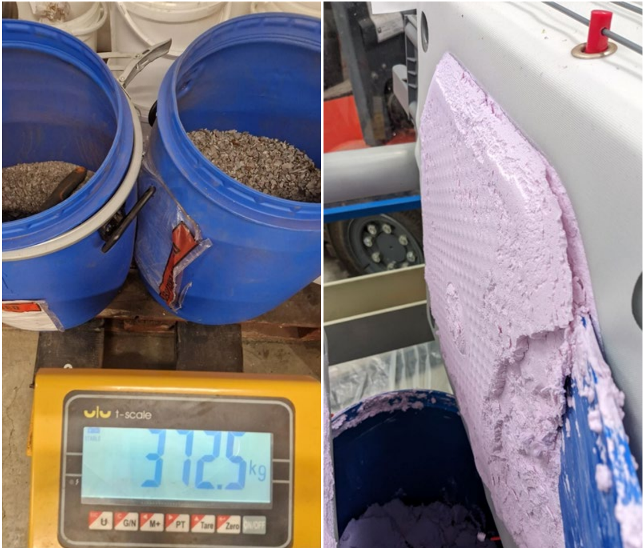
Figure 12: Left, crushed magnets prepared, and right, mixed rare earth filter cake prepared for downstream process commissioning activity.
