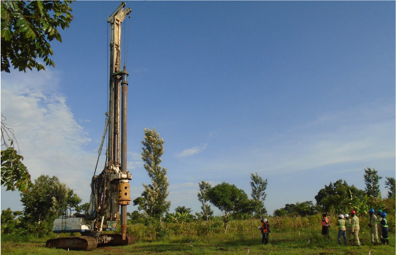
Figure 7: Auger drill mobilised to test site to collect bulk sample test material.
