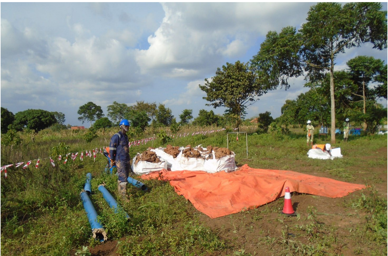
Figure 8: Bulk sample being collected for desorption column and crib metallurgical test work program.
