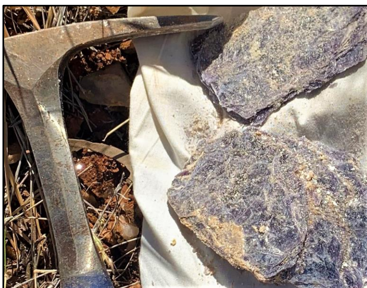
Figure 2: Examples of samples with high lithium and REE assays at QXR's Turner River, Pilbara. (Photo of sample collected in same location as 23QXRX-017 with 3.4% LiO2, with 50% mica, 30% feldspar, 20% quartz.)
