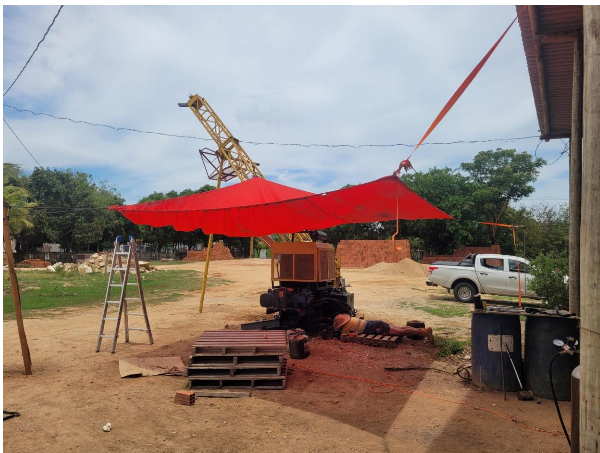
Figure 1: OzAurum diamond drill rig
