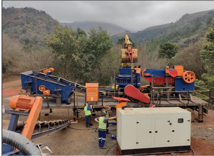
Figure 11: Crusher offloaded into position.
