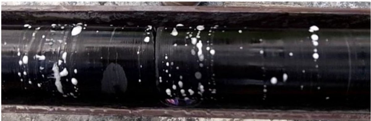
Figure 4: Gassy response from core sample at about 140m
