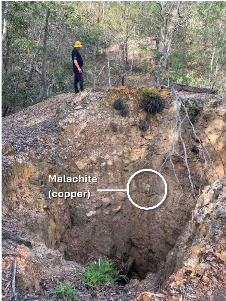
Figure 3. New shaft Identified 620m south-east of the old workings. Visible malachite in the wall of the shaft, with vertical depth of shaft estimated at 60m. (ASX Announcement 7 Sept 2023)
